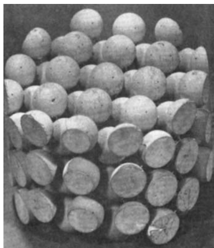
Fig. 1. Close-up view of distended, fixed bed in a body-centered cubic arrangement ( \epsilon = 0.576 ).
